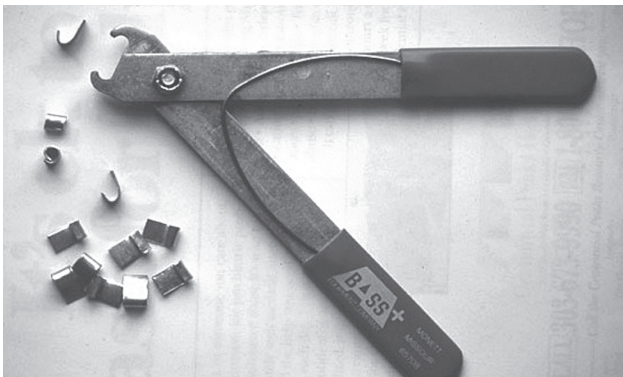
Figure 1. A basic set of crimping pliers with a handful of metal J-clips.
