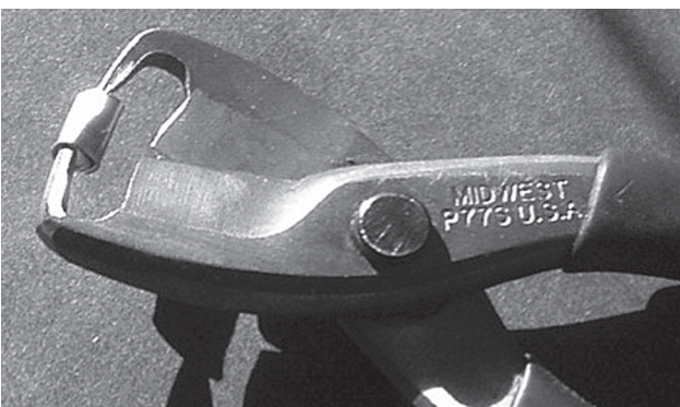
Figure 4. J-clip removal pliers easily remove a seated J-clip with a simple twist.
